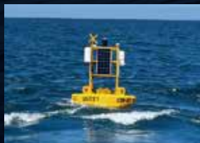
Velocity Observation (Sea Surface Installation)
